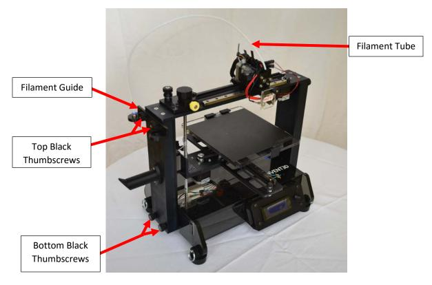
10. Connect the power supply by attaching it to the power plug on the back of the printer. Once that is complete, follow the procedure in the instructions on board leveling and z-axis calibration.
