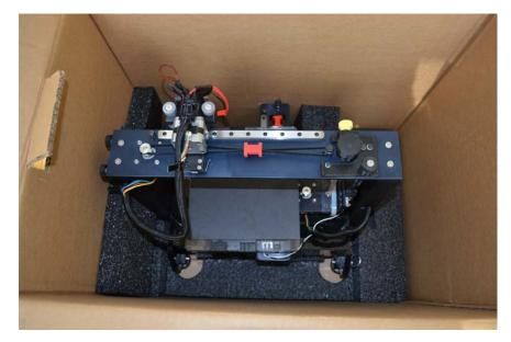
3. By grabbing both sides of the printer frame, lift the printer out of the box
